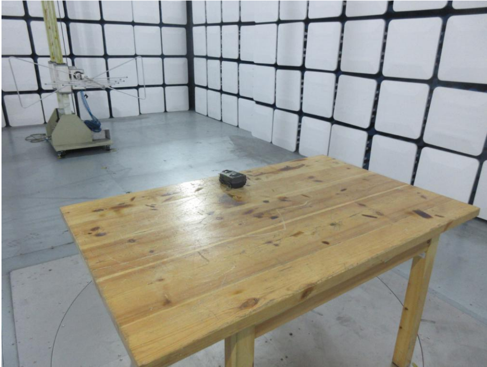
Photo of Radiation Emission Test
