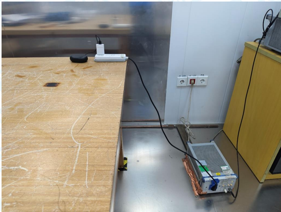
Photo of Setup for Conducted Emission
