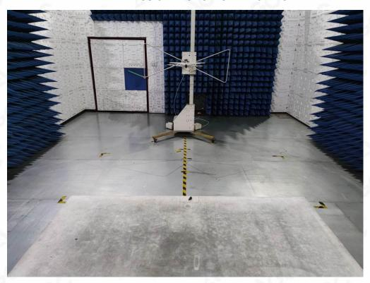
RADIATED EMISSION TEST SETUP ABOVE 1GHz
