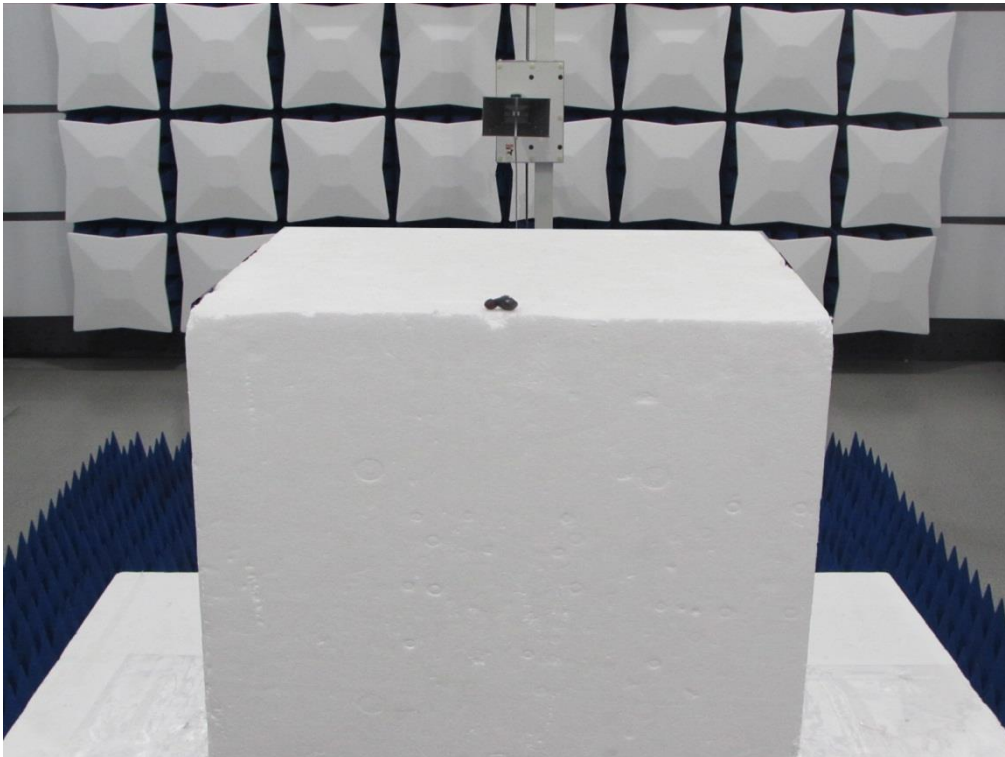
Radiated Emission Above 1GHz
