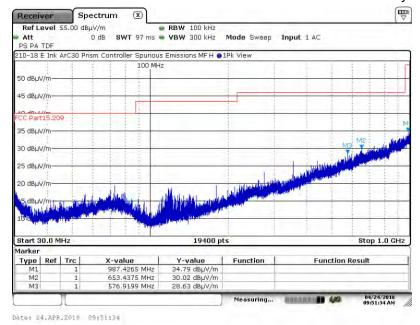
A3.2.2. Measurement Results: Vertical Receive Antenna Polarity
