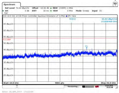
A7.1.2. Measurement Results: Vertical Receive Antenna Polarity
