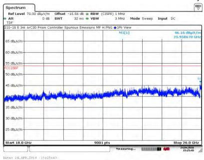
A7.2.2. Measurement Results: Vertical Receive Antenna Polarity
