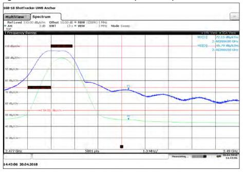
Band edge measurements were taken in real-time.
