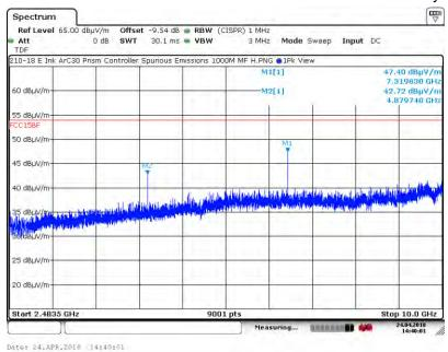
A5.2.2. Measurement Results: Vertical Receive Antenna Polarity
