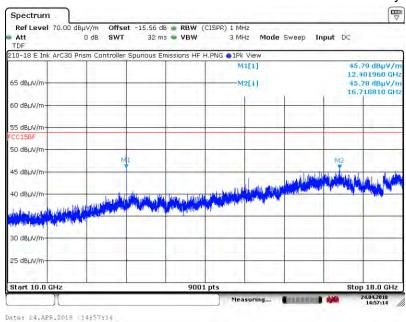
A6.3.2. Measurement Results: Vertical Receive Antenna Polarity
