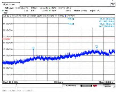
A6.2.2. Measurement Results: Vertical Receive Antenna Polarity
