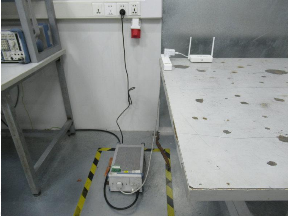
Photo of Conducted Emission Measurement
