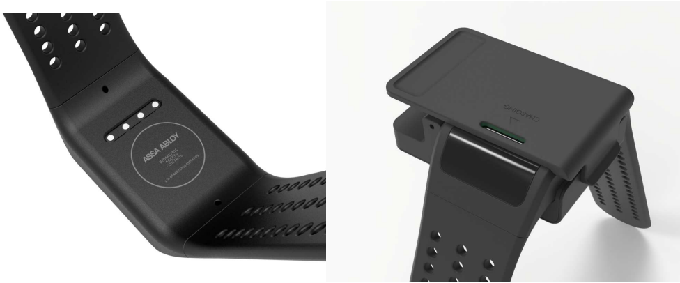
Figure 3: Wristband with pins for charging (left) and with charging clip attached (right)
