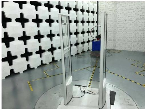
Radiated emission Test Setup-1 (30 MHz~1 GHz)
