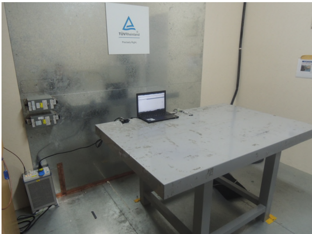
Photograph 9: Set-up for Mains Conducted testing Front
