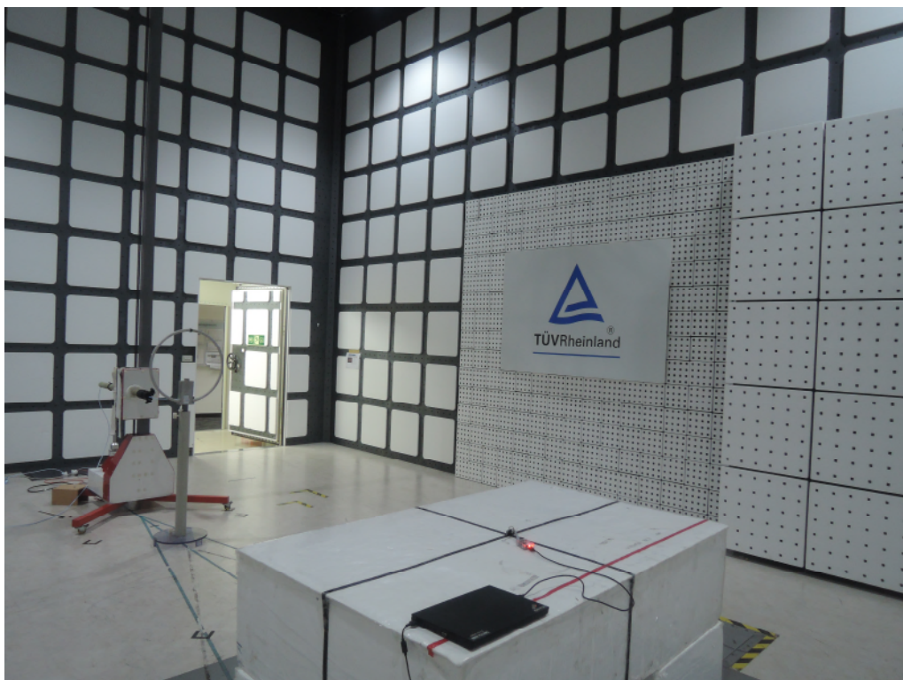
Photograph 5: Set-up for Spurious Emissions (Back View 3)
