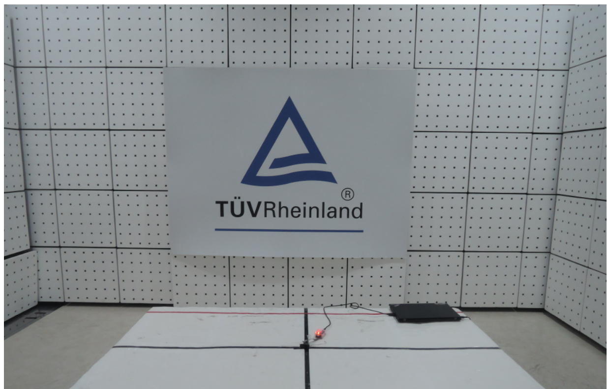
Photograph 1: Set-up for Spurious Emissions (Front View 1)
