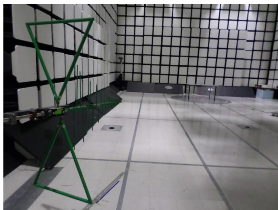
Figure 196: Radiated Spurious Emissions Test Setup, 30MHz-1000MHz - Setup Antenna View
