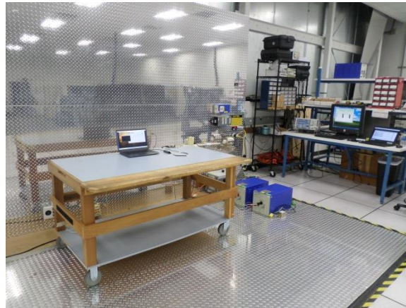
Figure 27: Conducted Emissions, Setup Front View
