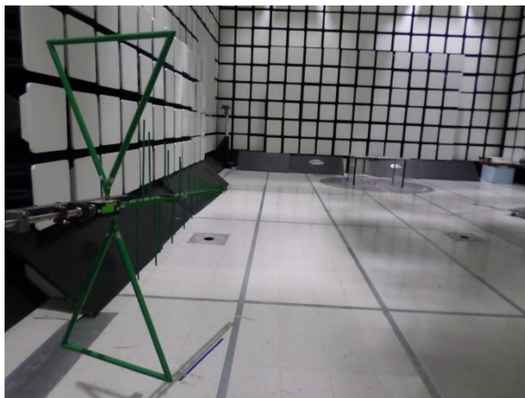
Figure 3: Radiated Spurious Emissions, 30MHz-1000MHz - Setup Antenna View
