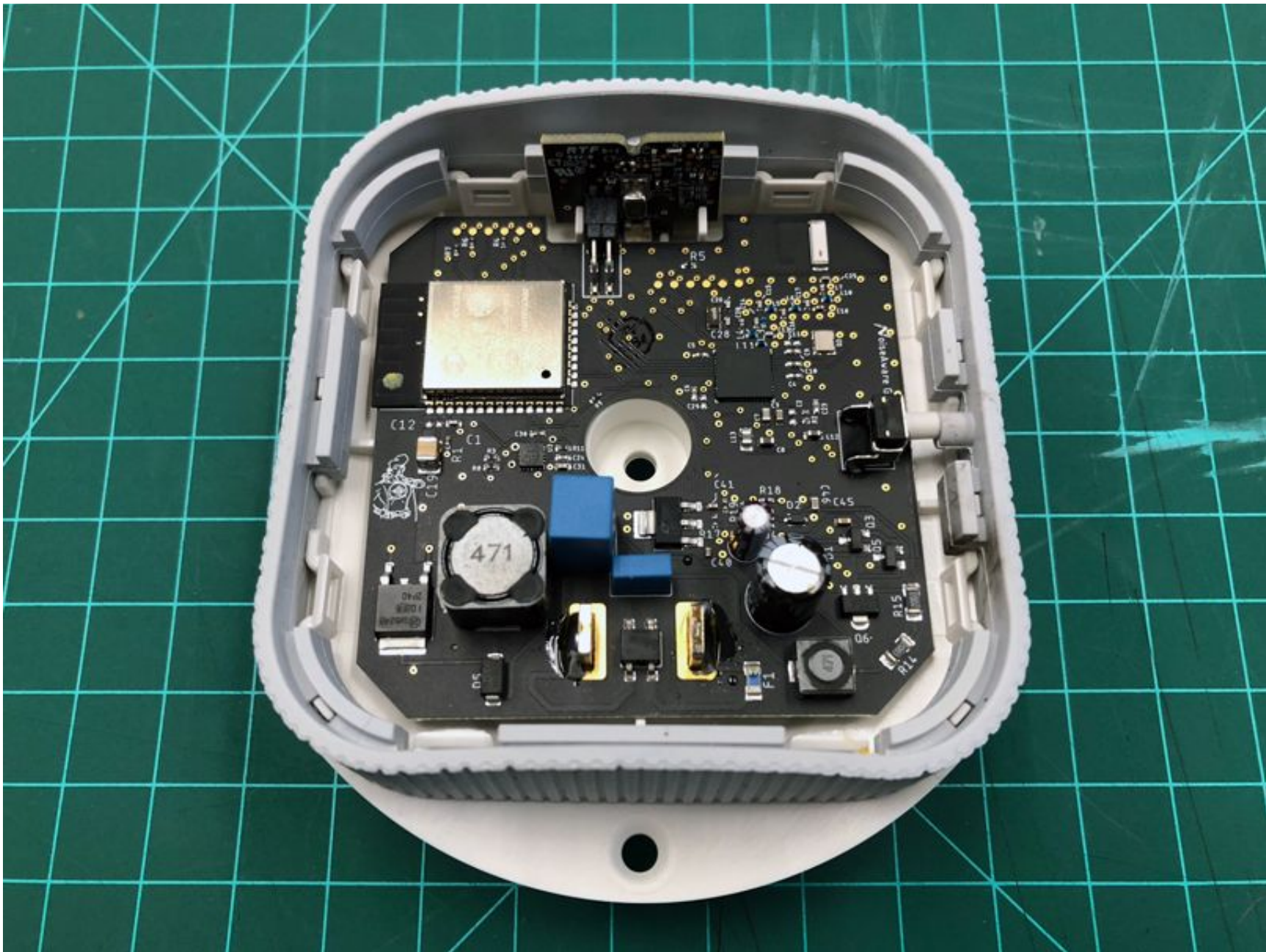
Gen3 Collector - Electronics Subassembly (shows placement of Main PCBA and Mic PCBA)
