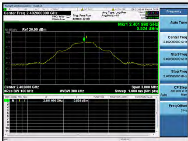
GFSK LOW CHANNEL, CARRIER LEVEL
