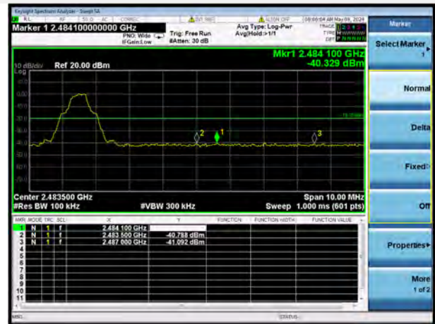
GFSK HIGH CHANNEL, BAND EDGE
