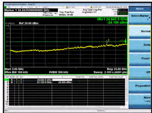
GFSK HIGH CHANNEL, SPURIOUS 3 GHz ~ 25 GHz
