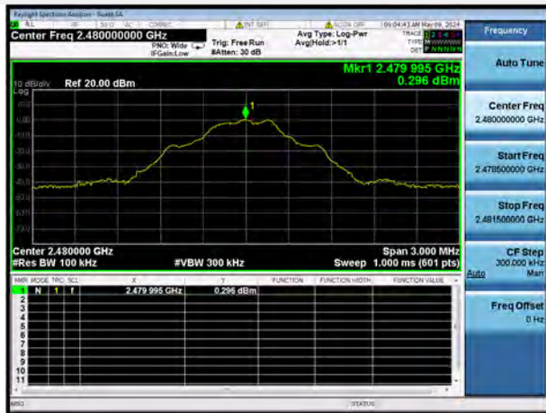
GFSK HIGH CHANNEL, CARRIER LEVEL
