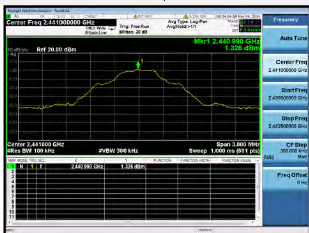
GFSK MIDDLE CHANNEL, CARRIER LEVEL
