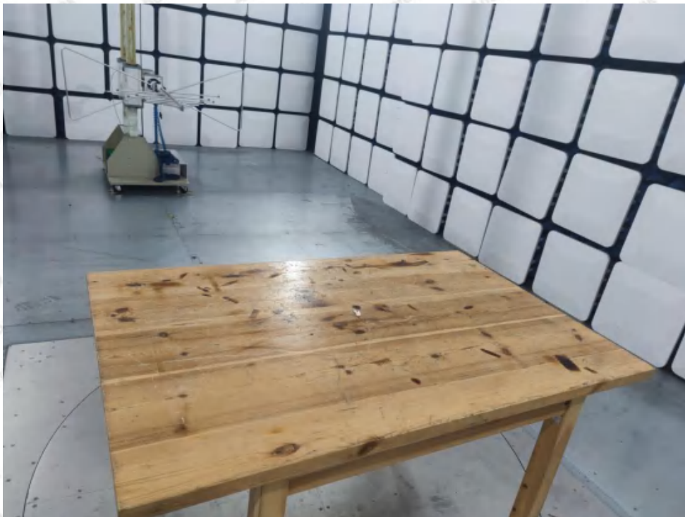
Photo of Radiation Emission Test
