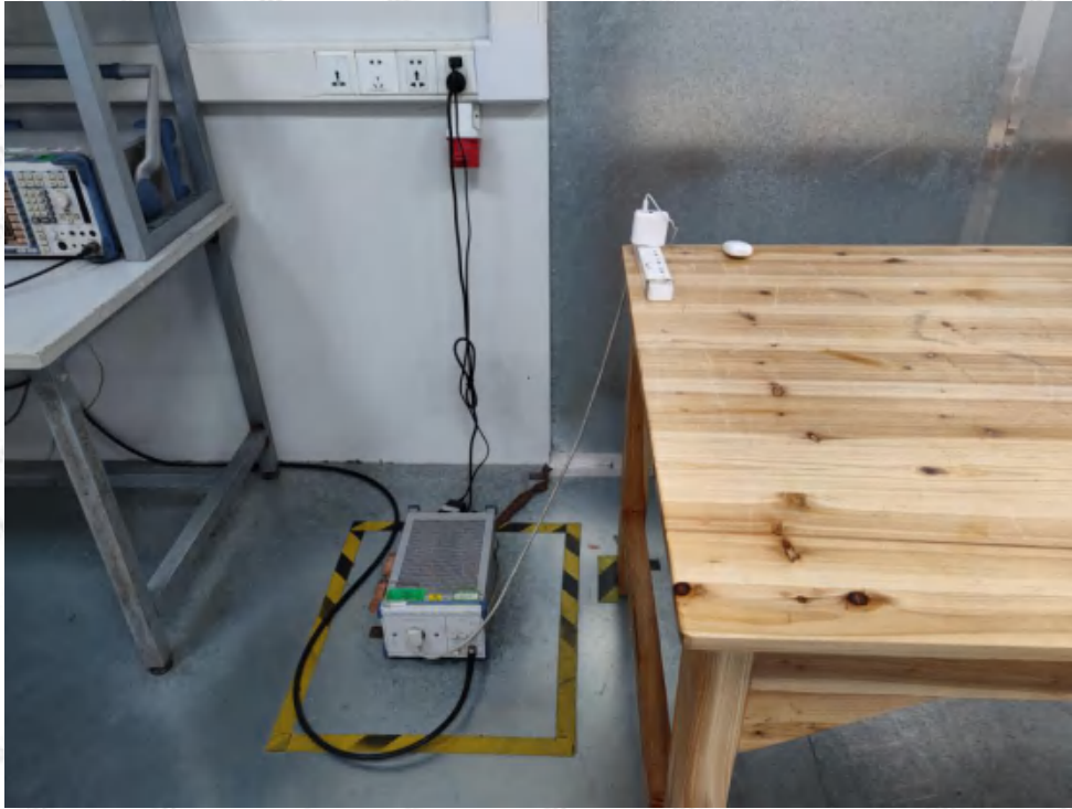
Photo of Conducted Emission Measurement
