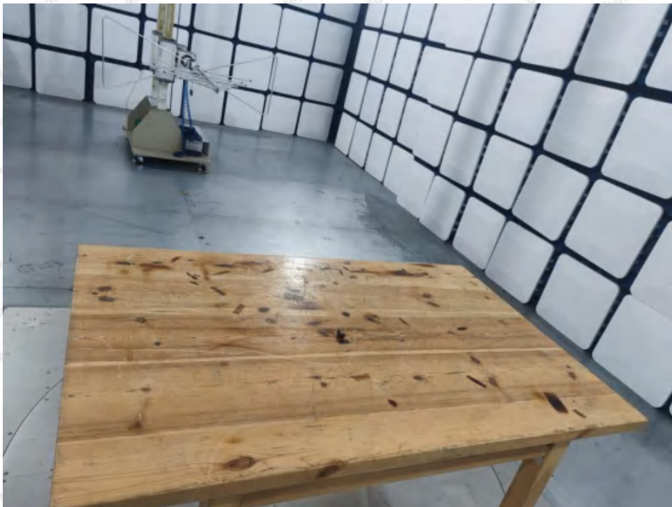
Photo of Radiation Emission Test
