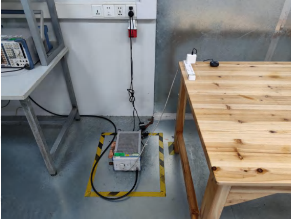
Photo of Power Line Conducted Emission Test
