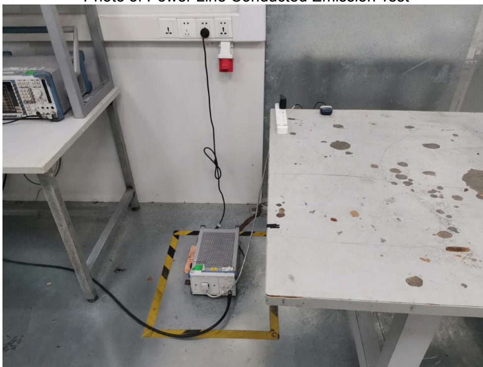
FCC ID: 2AQI5-WS105 Photo of Power Line Conducted Emission Test
