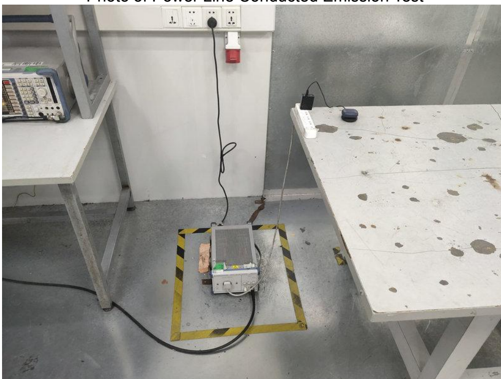
FCC ID: 2AQI5-WS105-CASE Photo of Power Line Conducted Emission Test
