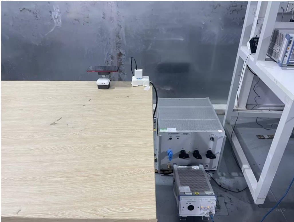
Conducted Emission-AC adapter charge mode
