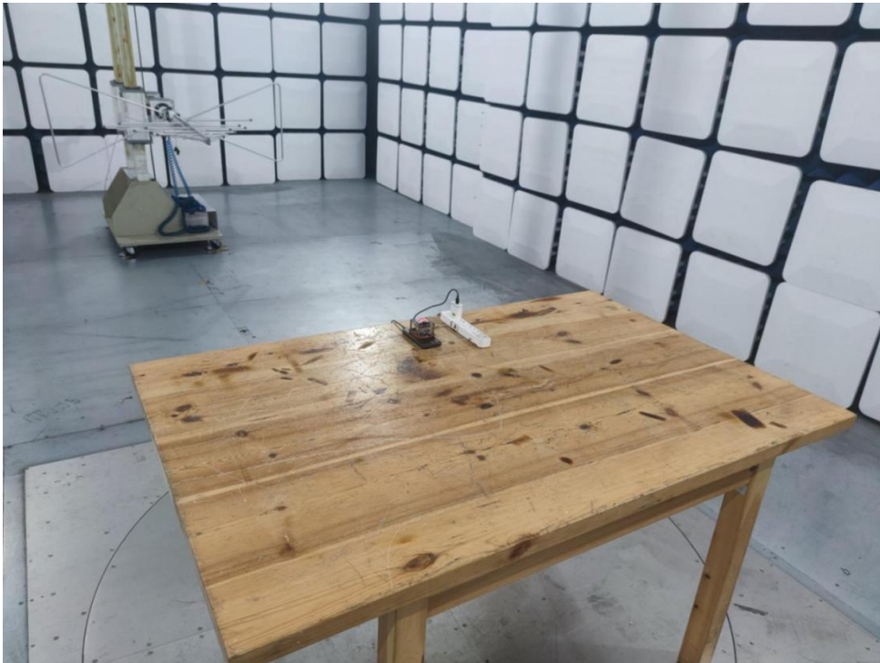
Photo of Radiation Emission Test
