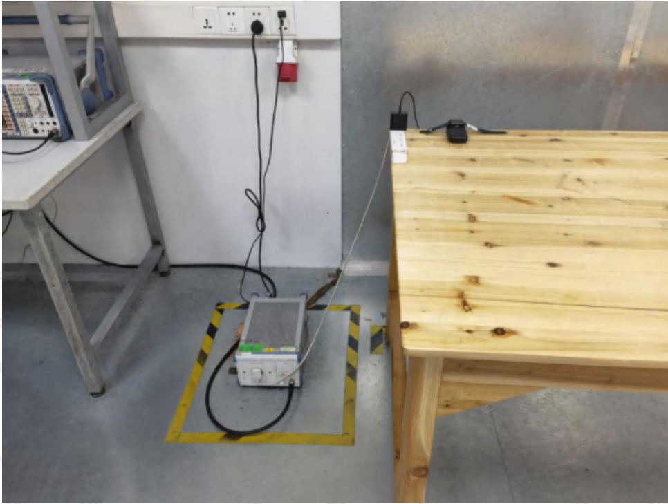
Photo of Conducted Emission Measurement
