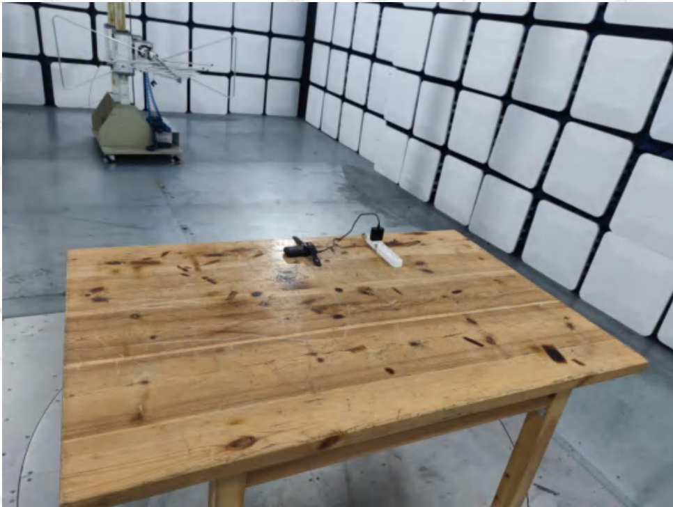
Photo of Radiation Emission Test
