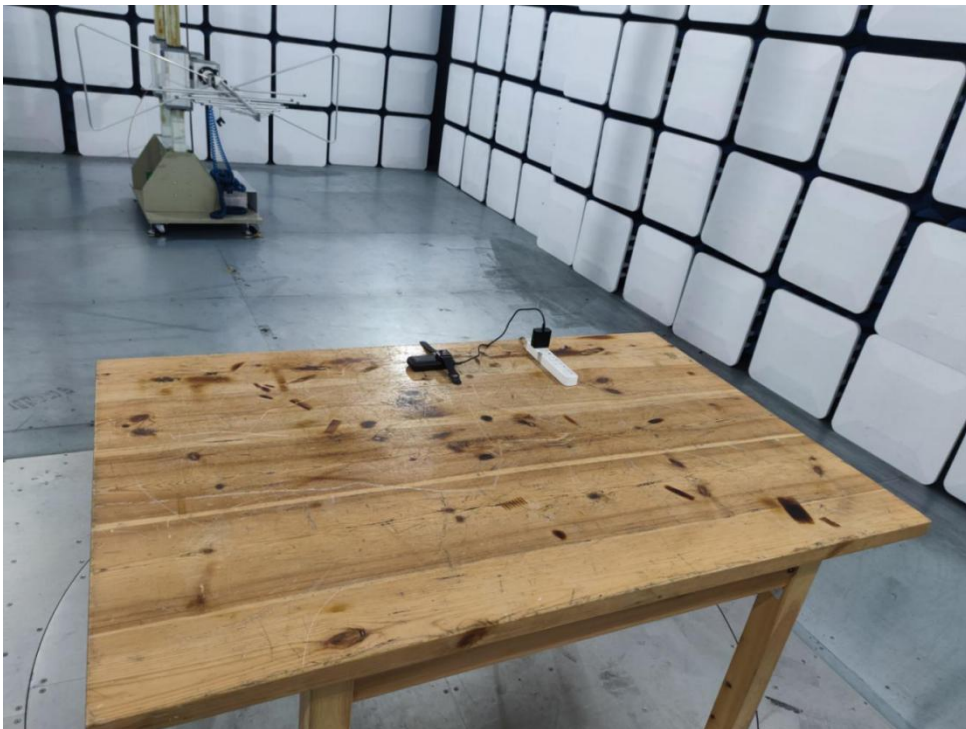
Photo of Radiation Emission Test
