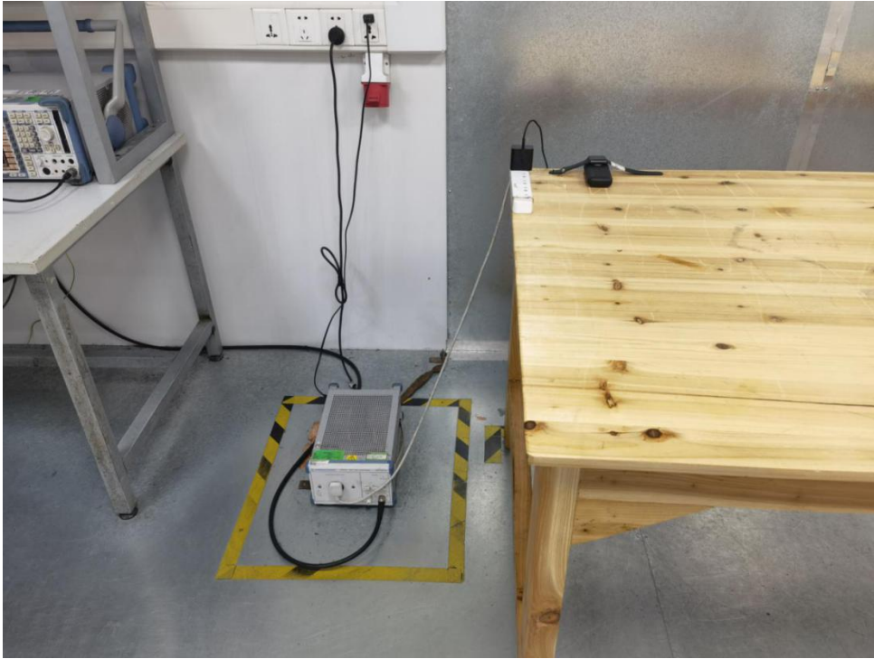
FCC ID: 2AQI5-PB111 Photo of Conducted Emission Measurement
