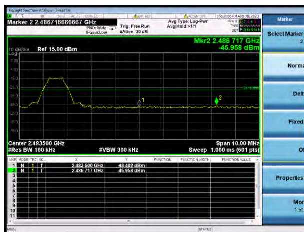
GFSK (BLE 1Mbps) HIGH CHANNEL, BAND EDGE
