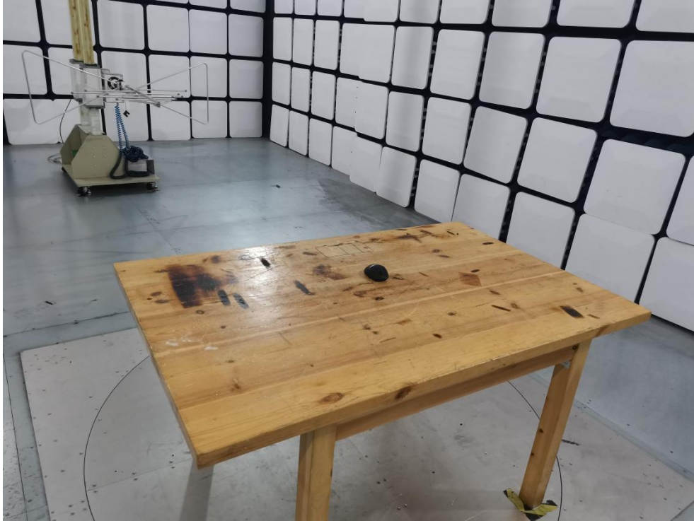
Photo of Radiation Emission Test
