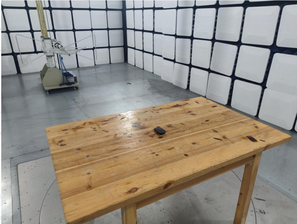
Photo of Radiation Emission Test
