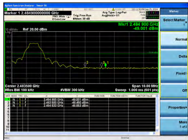
GFSK HIGH CHANNEL, BAND EDGE
