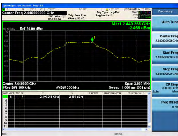
GFSK MIDDLE CHANNEL, CARRIER LEVEL
