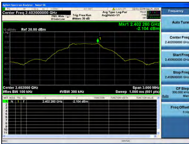
GFSK LOW CHANNEL, CARRIER LEVEL
