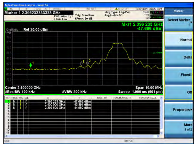
GFSK LOW CHANNEL, BAND EDGE
