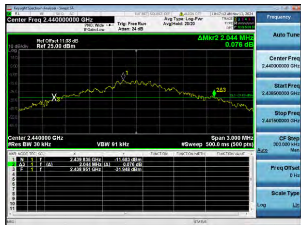
GFSK MIDDLE CHANNEL
