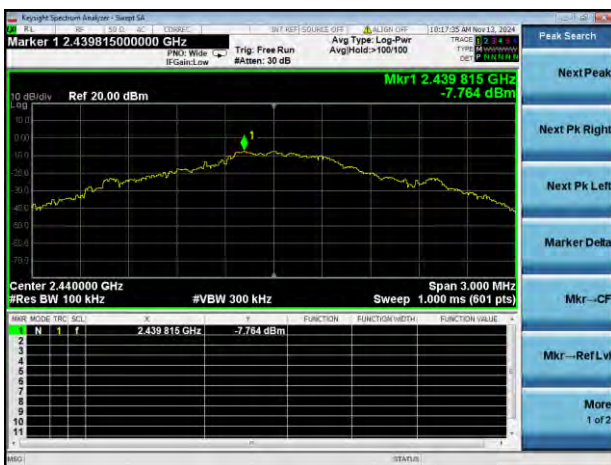
GFSK MIDDLE CHANNEL, CARRIER LEVEL
