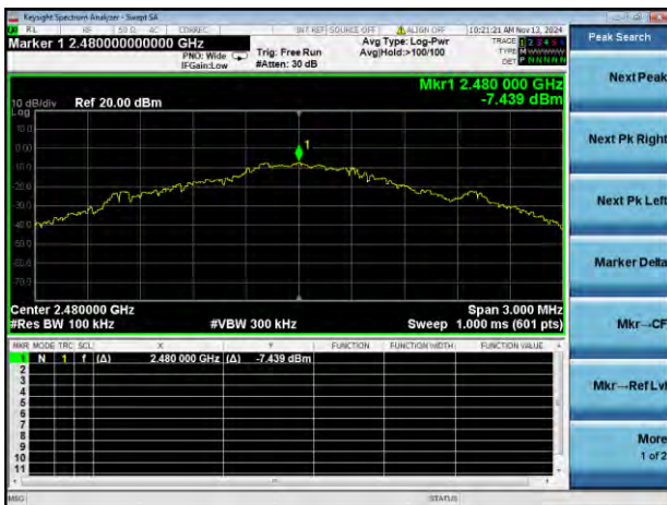
GFSK HIGH CHANNEL, CARRIER LEVEL
