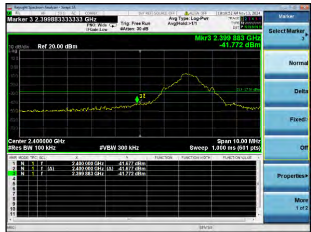
GFSK LOW CHANNEL, BAND EDGE
