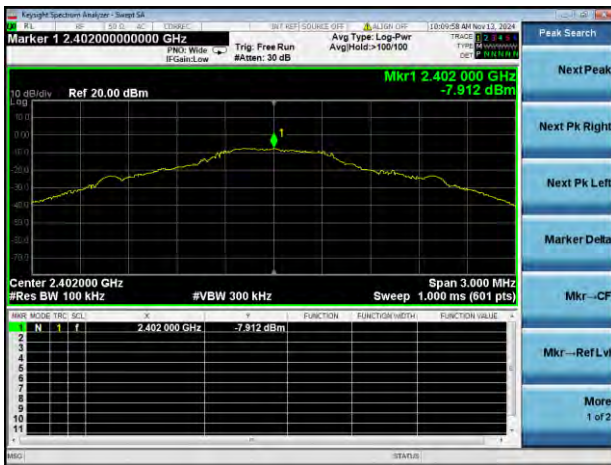
GFSK LOW CHANNEL, CARRIER LEVEL
