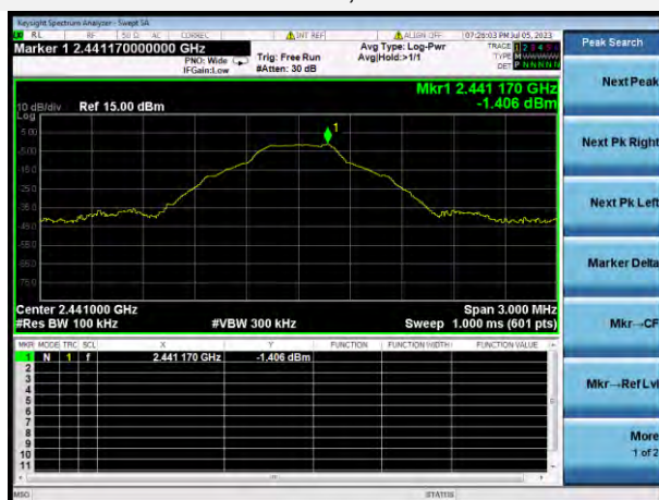
GFSK MIDDLE CHANNEL, CARRIER LEVEL
