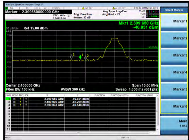
GFSK LOW CHANNEL, BAND EDGE
