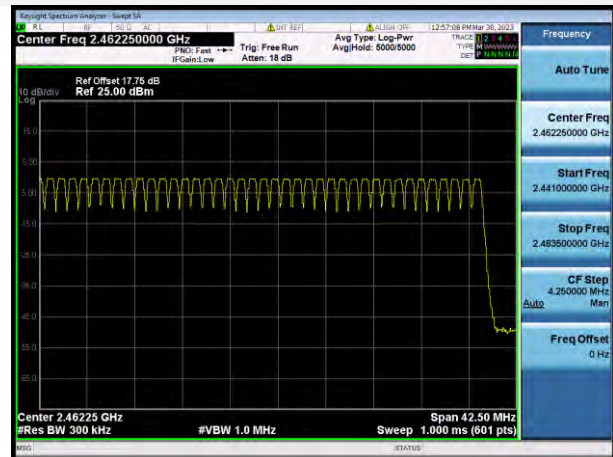
GFSK 2.4415 GHz ~ 2.4835 GHz
