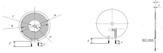
Note: Wrap 6MM (Min) high-temperature adhesive tape around the coil outlet position
