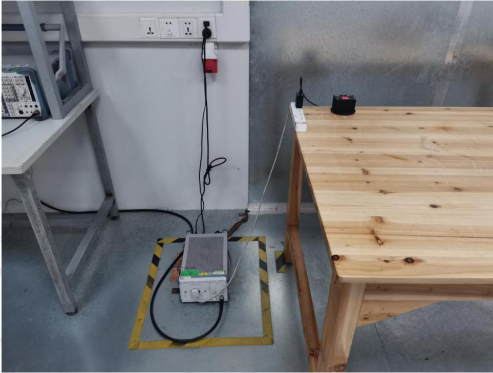
Photo of Conducted Emission Measurement
