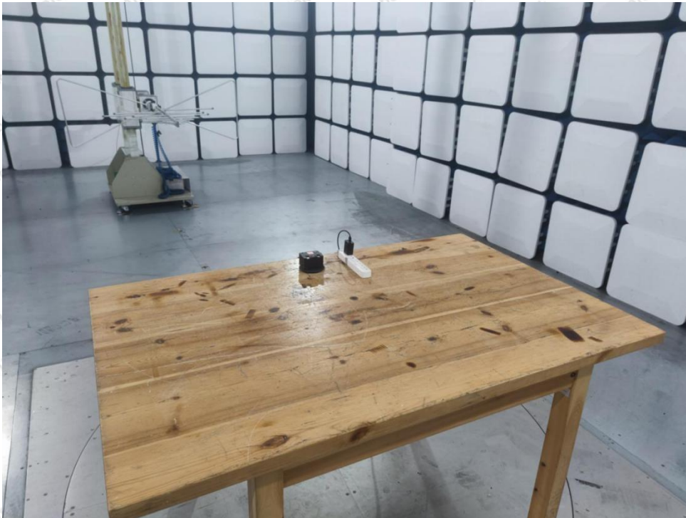
Photo of Radiation Emission Test
