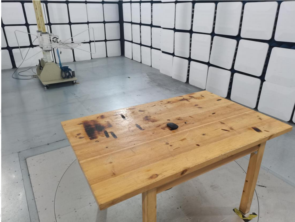
Photo of Radiation Emission Test
