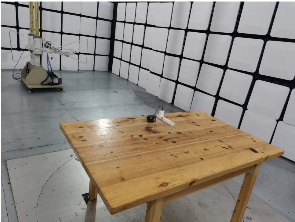
Photo of Radiation Emission Test
