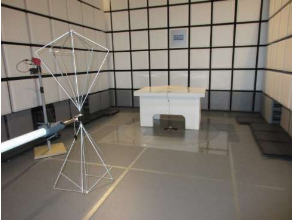
Figure 1: Radiated emission test
