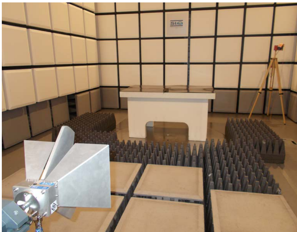
Figure 7: Radiated emission test – 1000 MHz – 6000 MHz (without charger)
