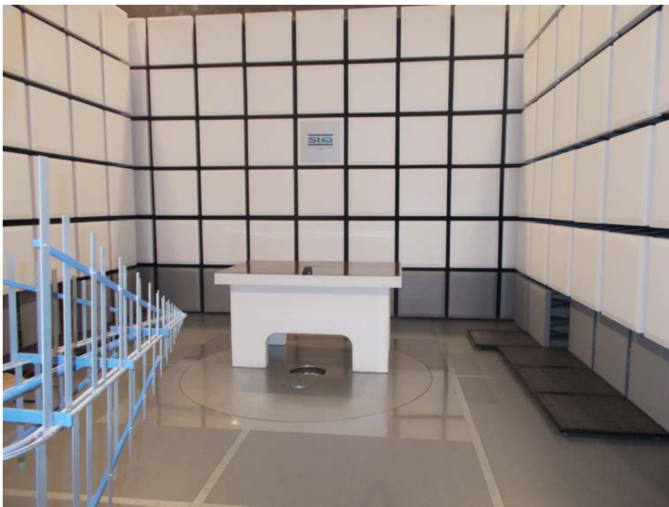
Figure 5: Radiated emission test – 200 MHz – 1000 MHz (without charger)
