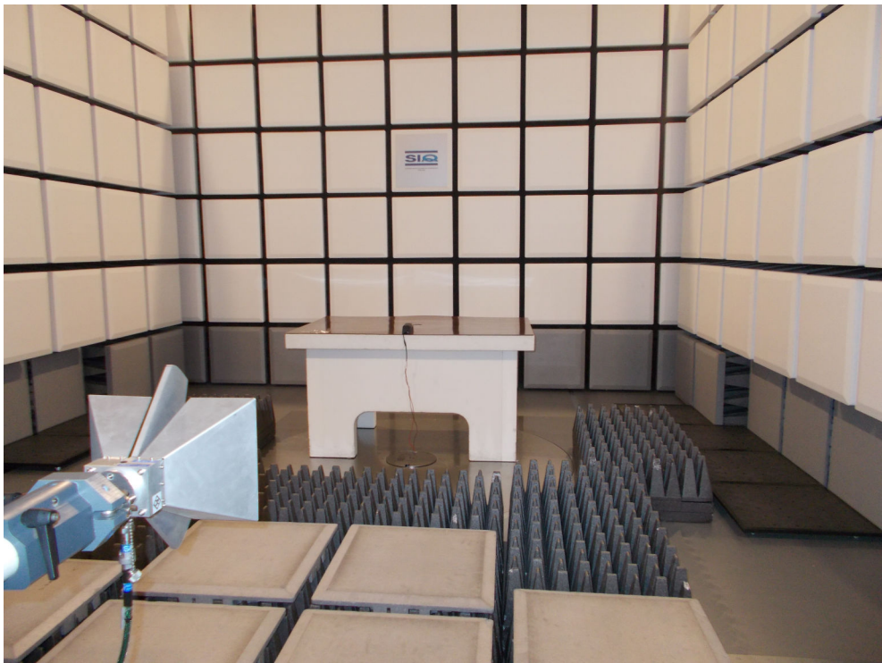
Figure 9: Radiated emission test – charging from battery power supply
