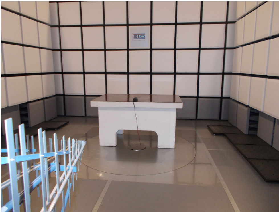
Figure 6: Radiated emission test – charging from battery power supply
