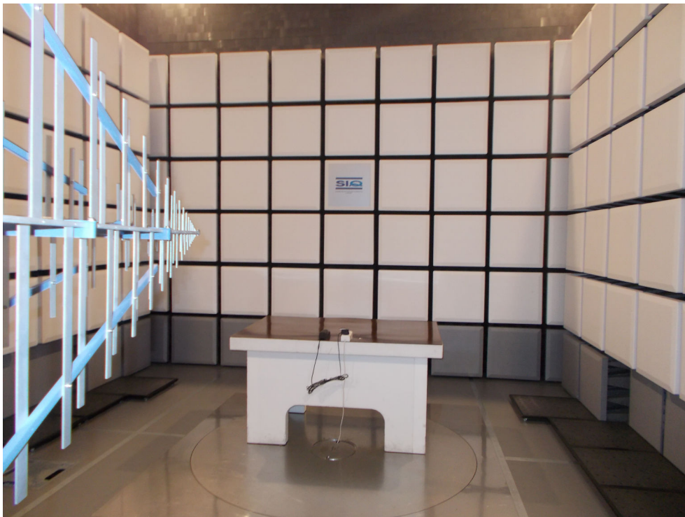
Figure 7: Radiated emission test – charging from AC/DC power supply
