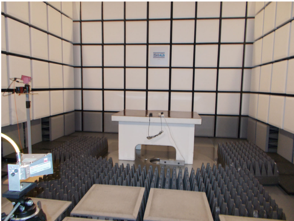
Figure 13: Radiated emission test – charging from AC/DC power supply
