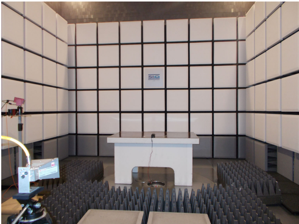
Figure 12: Radiated emission test – charging from battery power supply
