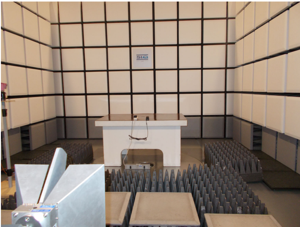
Figure 10: Radiated emission test – charging from AC/DC power supply
