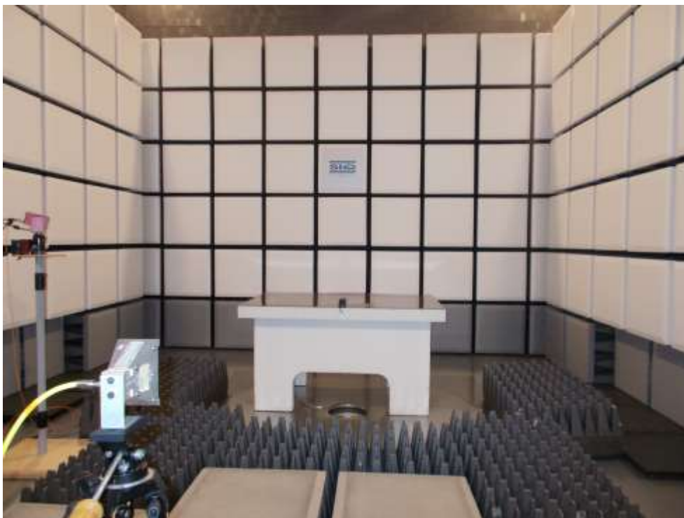
Figure 11: Radiated emission test – battery operating
