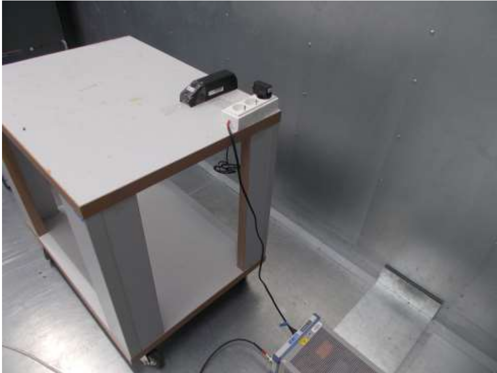
Figure 1: Conducted emission test – Charging from AC/DC power supply
