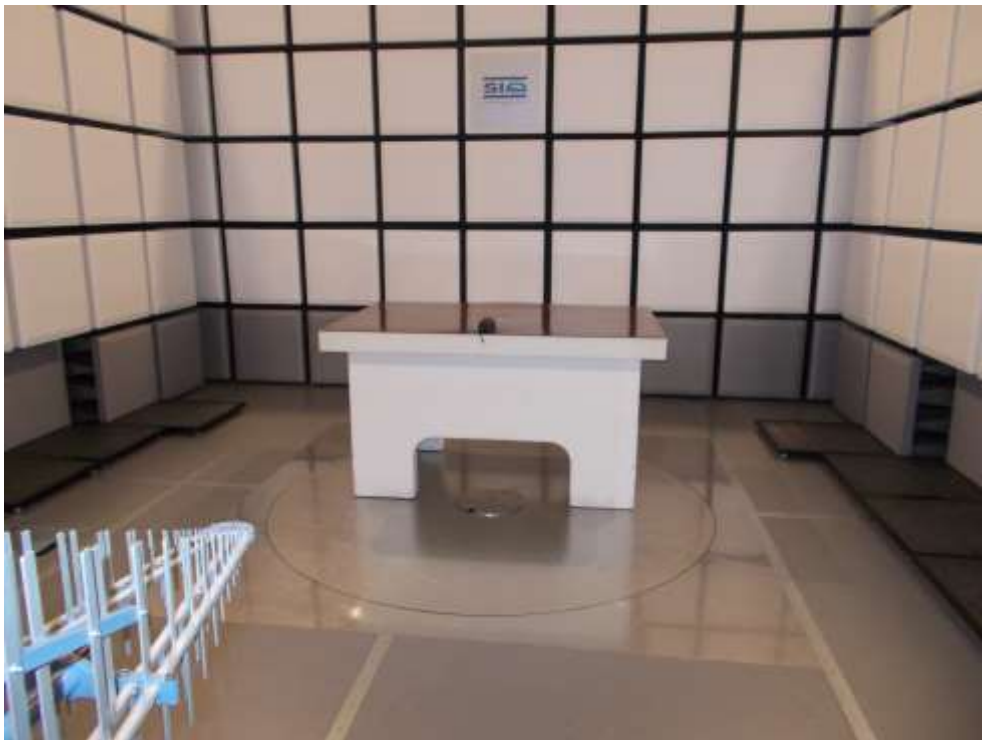
Figure 5: Radiated emission test – battery operating
