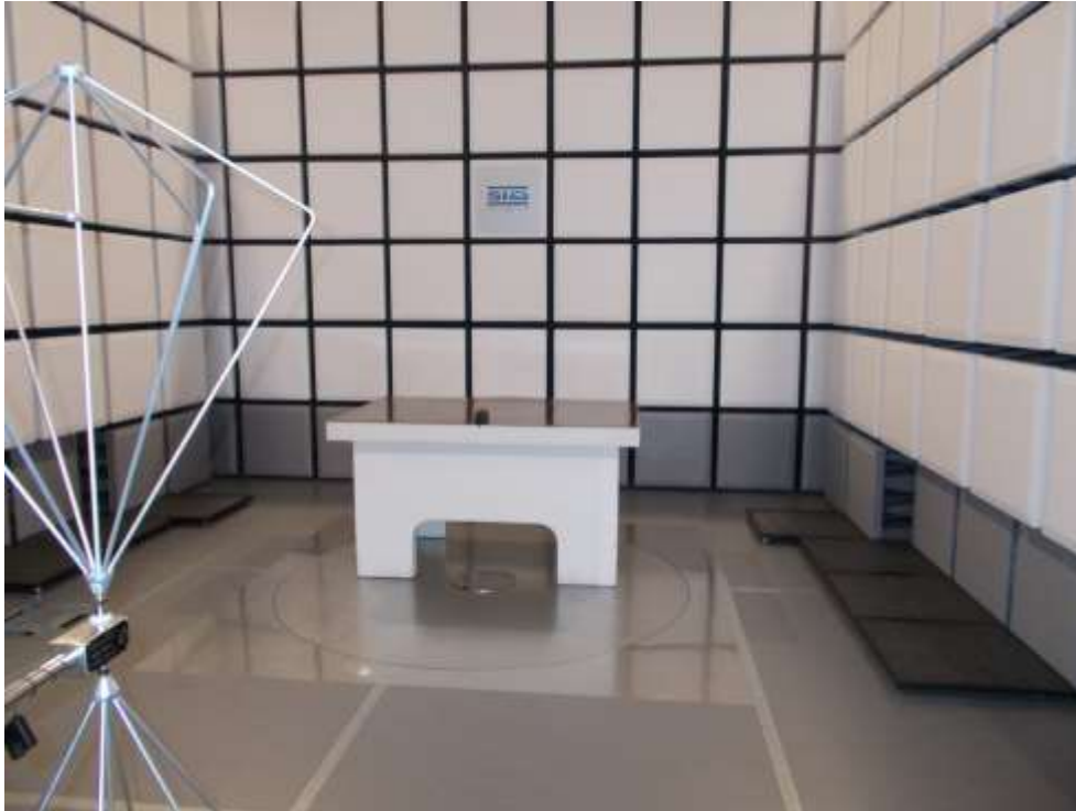
Figure 2: Radiated emission test – battery operating
