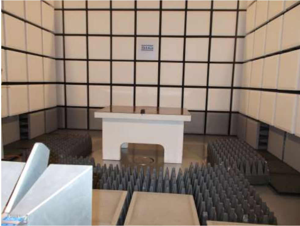
Figure 8: Radiated emission test – battery operating
