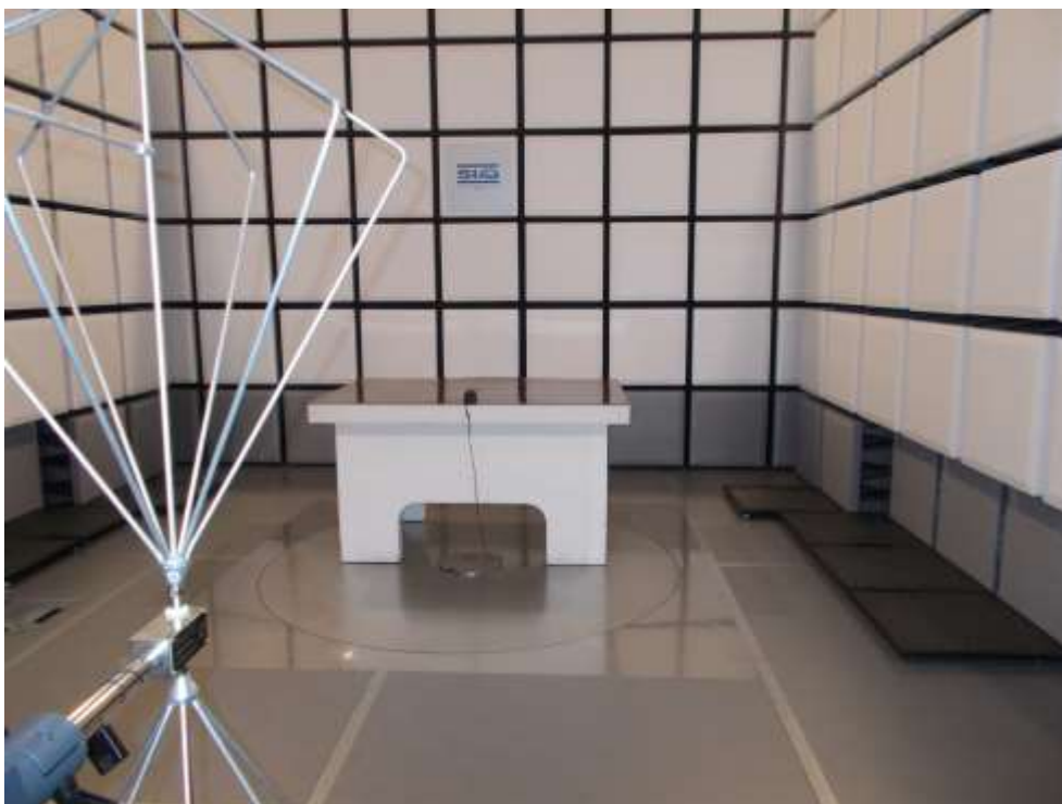
Figure 3: Radiated emission test – charging from battery power supply
