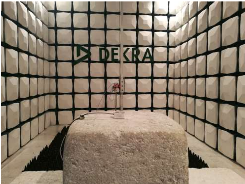
Description: Radiated Emission Test Setup for 1~18GHz
