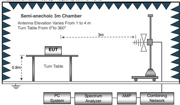
(C) Radiated Emission Test-Up Frequency Above 1GHz
