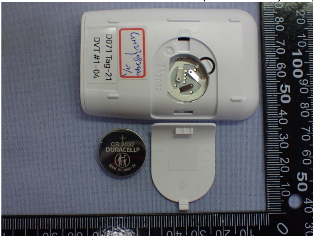
Internal View (Removed Battery Cover)
