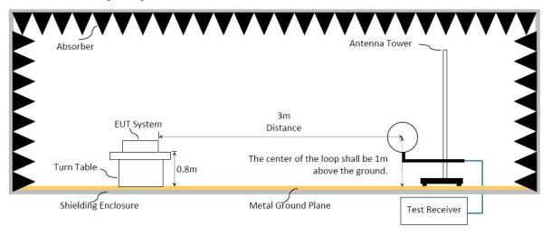
6.1.3. Setup Diagram for 30-1000 MHz
