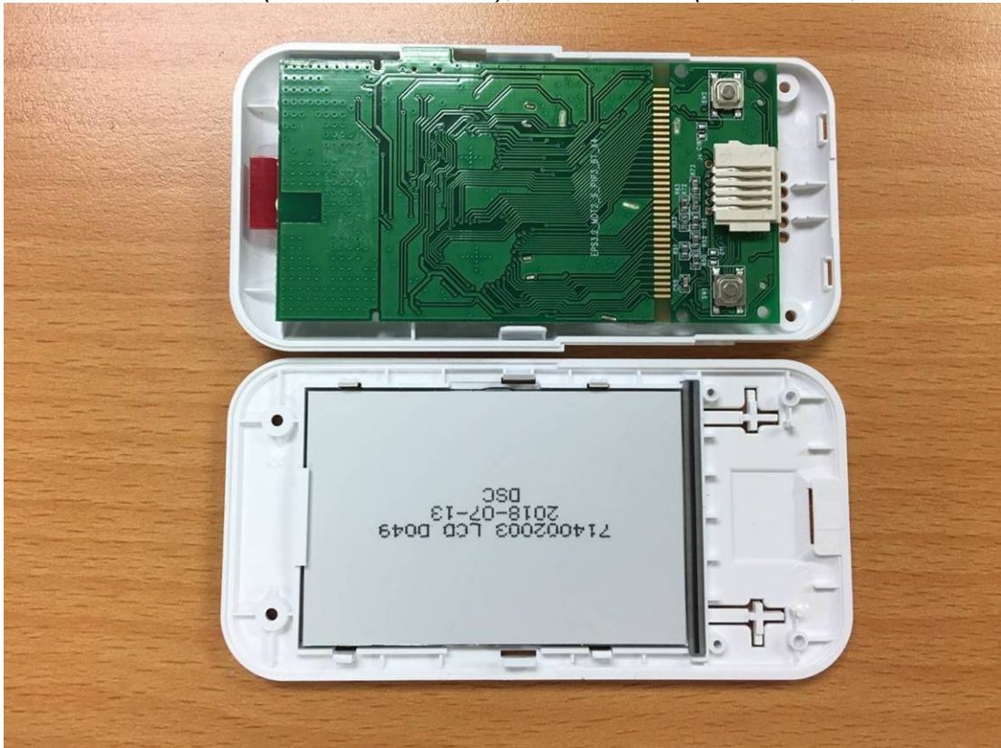
Figure 25 MDT2 BLE (with FDA Version), Internal View (Main Board, Back View)
