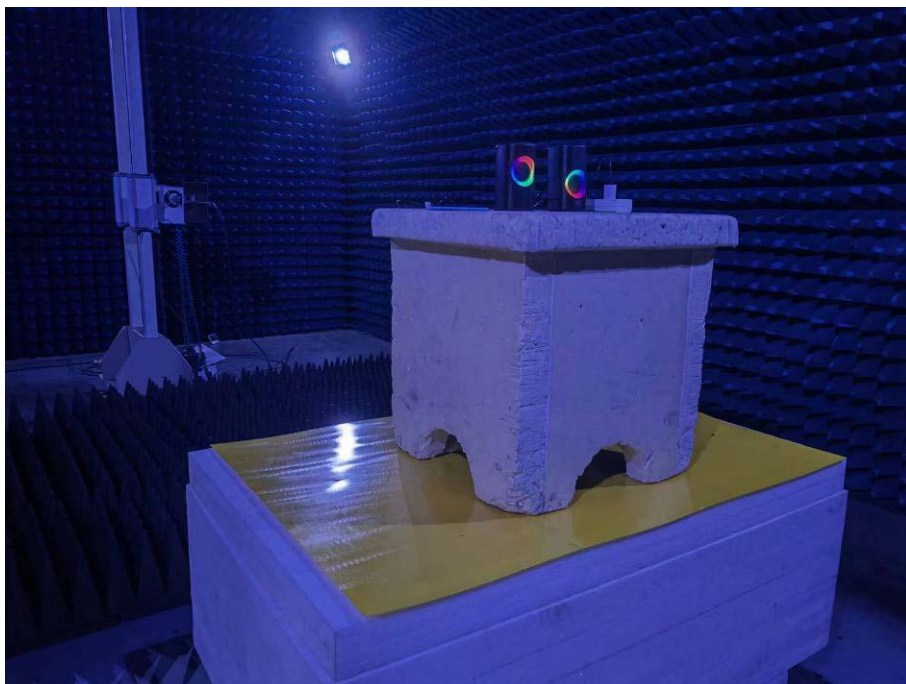
Photo of Radiated Emission Measurement Above 1GHz
