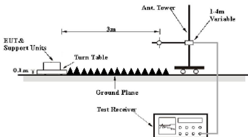
The radiated emission below 1GHz tests were performed in the 3 meters chamber A, above 1GHz tests were performed in the 3 meters chamber B, using the setup accordance with the ANSI C63.10-2013. The specification used was the FCC 15.209, and FCC 15.247 limits.
