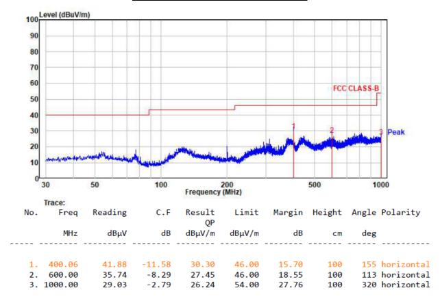
Remarks: C.F (Correction Factor) = Antenna factor + Cable loss - Preamp gain
