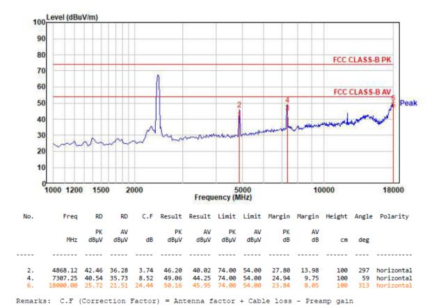
100 Level (dBuV/m) 90 80 FCC CLASS-B PK 70 60 FCC CLASS-B AV 50 Peak 40 30 20 10 1000 1200 1500 2000 5000 10000 18000 Frequency (MHz) Freq RD RD C.F Result Result Limit Limit Margin Margin Height Angle Polarity No. PK ΑV PK PK ΑV PK ΑV ΑV  $dB\mu V \\$  $dB\mu V$ MHz dBuV dBuV dB dΒμV dBuV dB dB cm deg 4868.12 36.92 32.76 3.74 40.66 36.50 74.00 54.00 33.34 17.50 100 0 vertical
