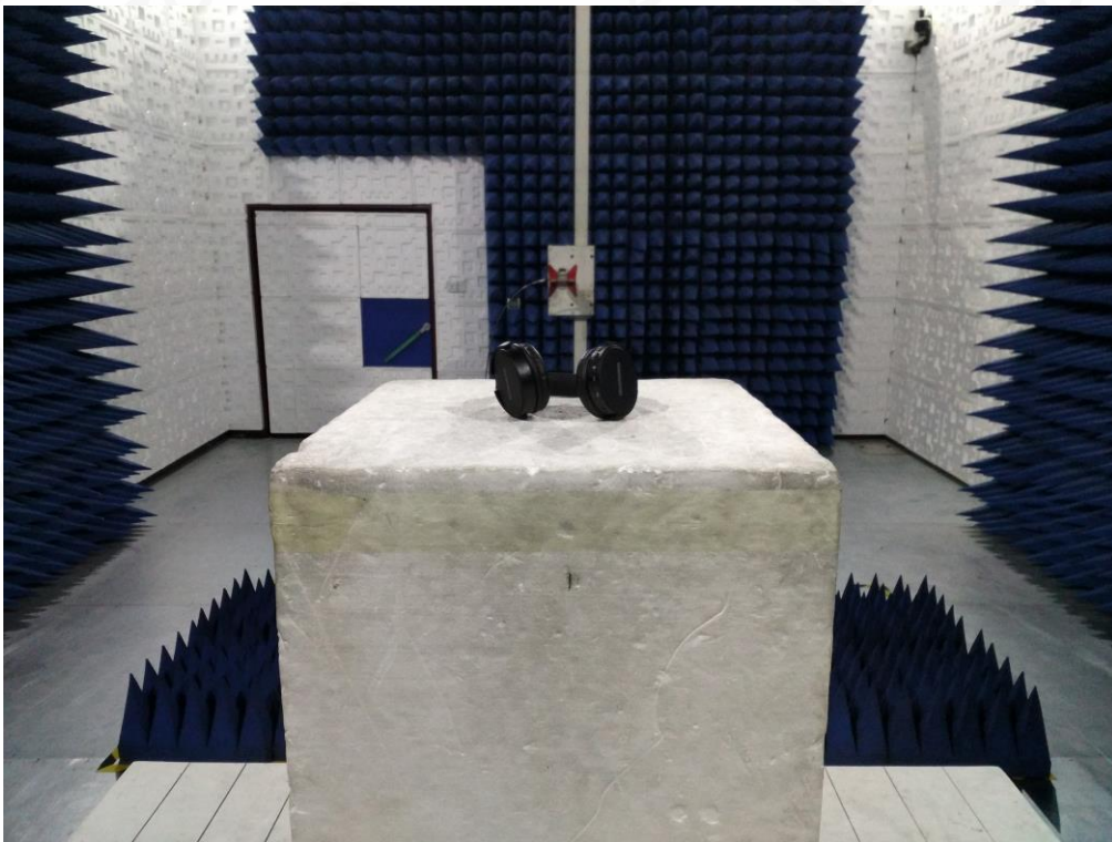
RADIATED EMISSION TEST SETUP ABOVE 1GHZ
