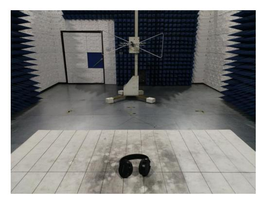
RADIATED EMISSION TEST SETUP ABOVE 1GHZ
