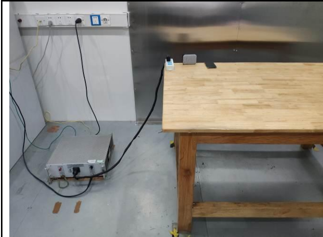
Conducted Emissions Test Setup Front View
