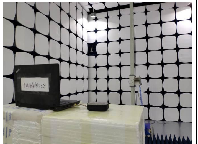
Radiated Spurious Emissions Test Setup Above 1GHz
