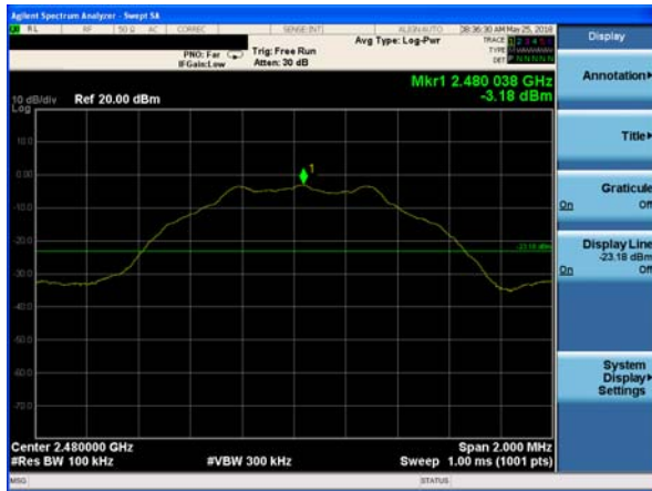
GFSK on channel 39
