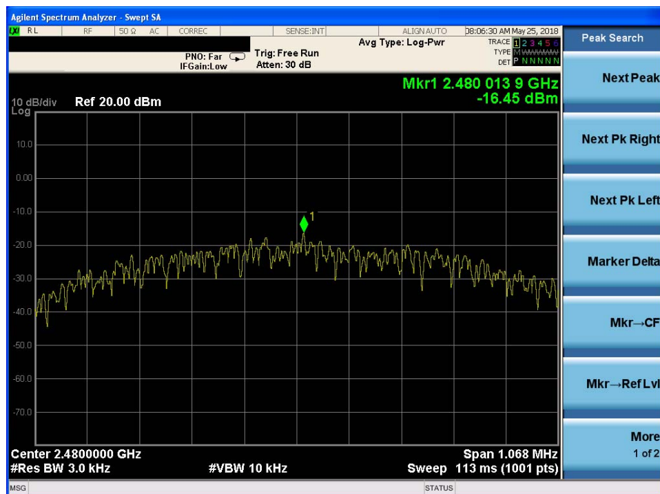
Power spectral density plot on channel 39
