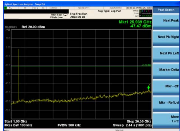
GFSK on channel 19
