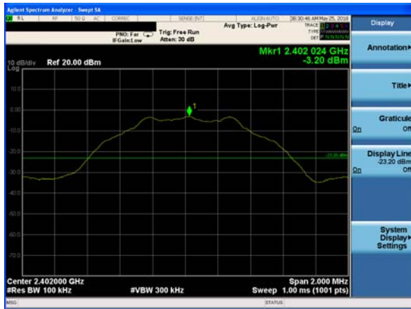
GFSK on channel 00
