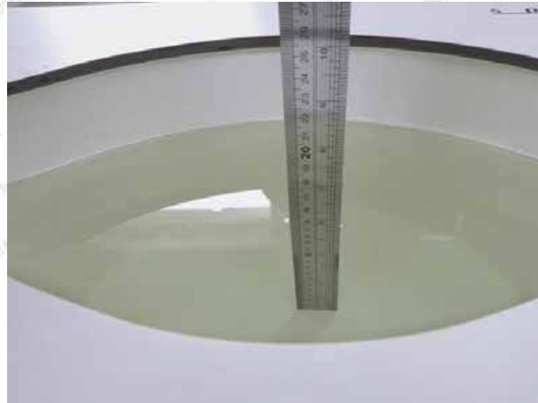
Liquid depth in the body phantom (2450MHz)
