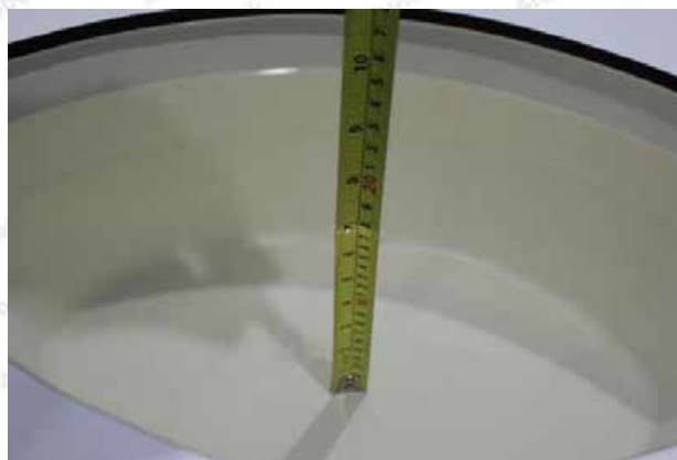
Liquid depth in the body phantom (5GHz)
