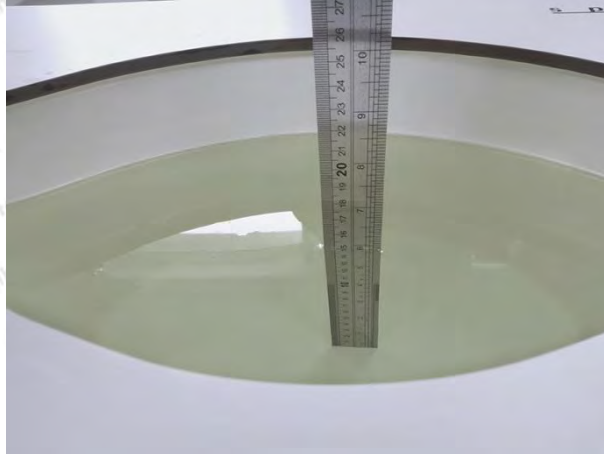
Liquid depth in the body phantom (2450MHz)
