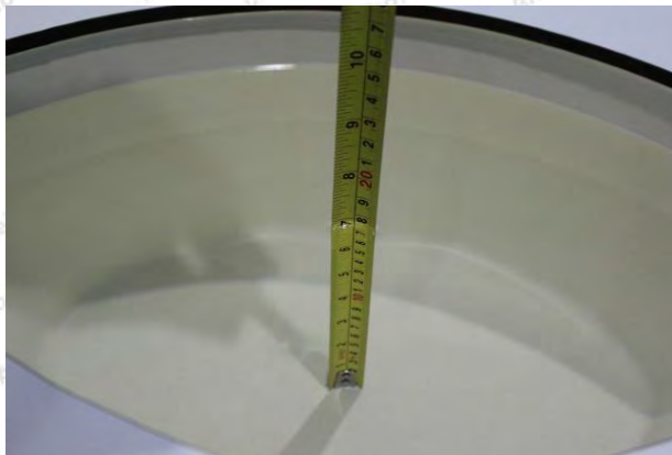
Liquid depth in the body phantom (5GHz)
